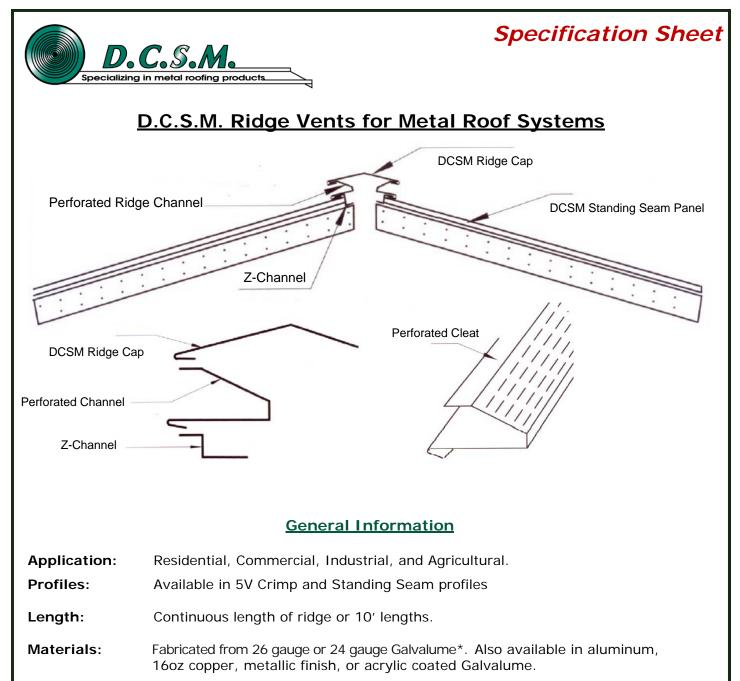
**Colors:** Available in all DCSM standard Colors. Roof panels and accessories are fabricated from the same coil stock as the ridge vent.
